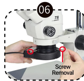
LED Light Installation
