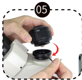
Synchronous Port Assembly
